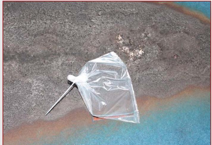
Recovery of carpet sample for ignitable liquid residue analysis
