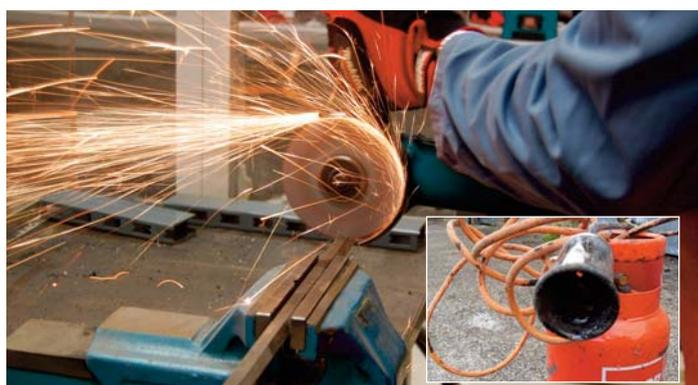
The hazards posed by hot work are well known and it is advised that it should only be carried out when other methods have been considered first. In some industries, hot work is part of the day to day process and permanent hot work areas are provided, constructed from suitably non-combustible materials with the necessary precautions 'built in'.
